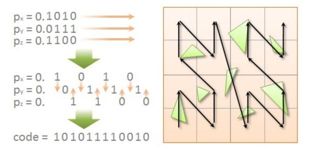
The Z-order curve is defined in terms of *Morton codes*. To calculate a Morton code for the given 3D point, we start by looking at the binary fixed-point representation of its coordinates, as shown in the top left part of the figure. First, we take the fractional part of each coordinate and expand it by inserting two "gaps" after each bit. Second, we interleave the bits of all three coordinates together to form a single binary number. If we step
